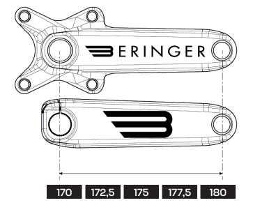
CrMo integrated steel shaft with 24 mm diameter and steel pedal notches
